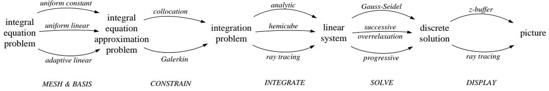
Figure 12: Steps of finite element simulation of radiosity.
